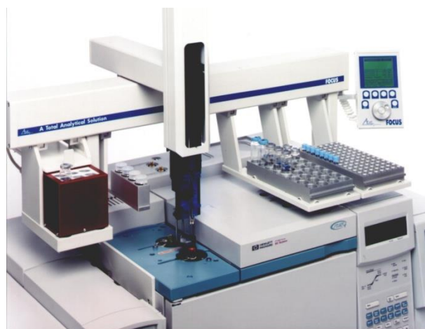
ATAS FOCUS Sample Processing Robot on HP6890
